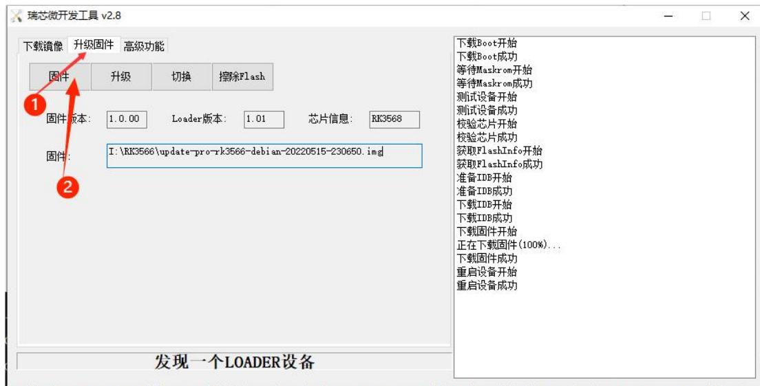
6. After loading is complete, click "**擦除 Flash(Erase Flash)**" , Once a confirmation dialog appears, it means the erase is successful.
