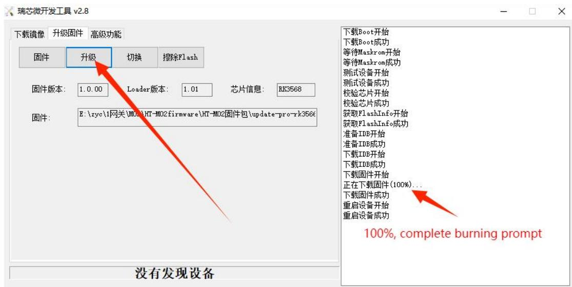
8. Device will reboot. Allow it to cool for 2-3 minutes before disconnecting the power. Press the **REC** button, don't release, then powering on, until RKDevTool will display "发现一个 **LOADER** 设备 (**Loader device detected**)", release the **REC** button.
